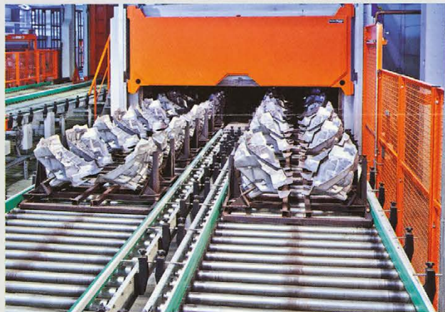
Aluminium suspension-strut supports in FINOBA's heat treatment plant
