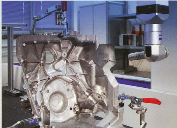
Coordinate-measuring machine for components up to 2,400 mm long
