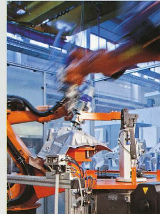
Automated assembly of wire thread inserts at the Baunatal plant
